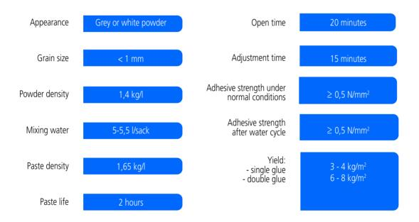
Data based on tests carried out under normal laboratory conditions 23  $\pm$  2°C and 50  $\pm$  5%HR < 0.2 m/s
